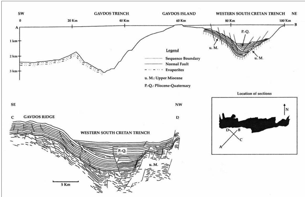
Figure 28. Example from the six backstop basins southward of Crete (Gavdos, Gortys, Poseidon, Ptolemeus, Pliny and Stravon trenches). Interpretation of seismic reflection profiles across the western south Cretan Trench. P.Q. recent sedimentary cover. uM, Miocene evaporite and related tectonics, Maravelis et al., 2012.
