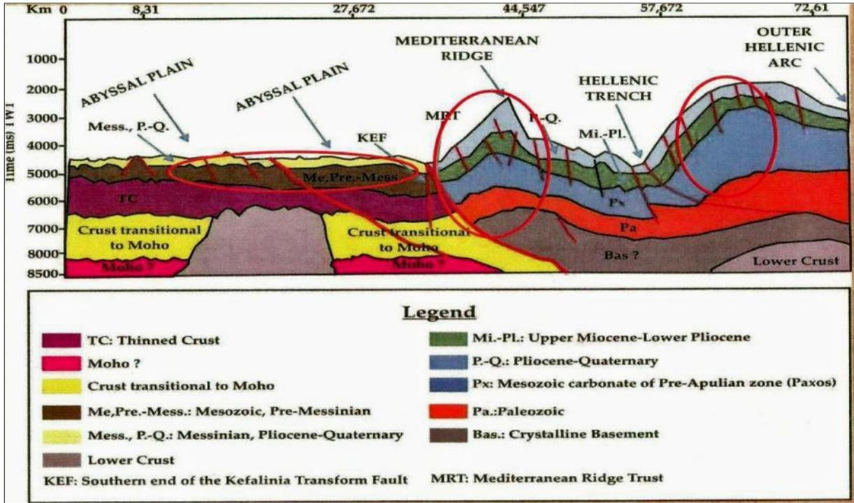
Figure 27. Possible hydrocarbon plays offshore southern Crete. Two major anticlines (ellipsoidal red circles) and the Hellenic trench, 2 Km below sea level. Also, Abyssal Plain (Oval red Circle). Zeliidis, 2011.
