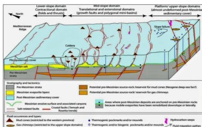
Figure 17. Active Mud Flow Volcanoes (brown triangles), Gas chimneys (brown discs), and Thermogenic Pockmarks and Mounds offshore Southern Crete. The pre-Messinian source rocks/ reservoir for the mud cones (brown), are highly visible as well as the reservoir/source for the gas chimneys (light brown), Loncke et al., 2004.
