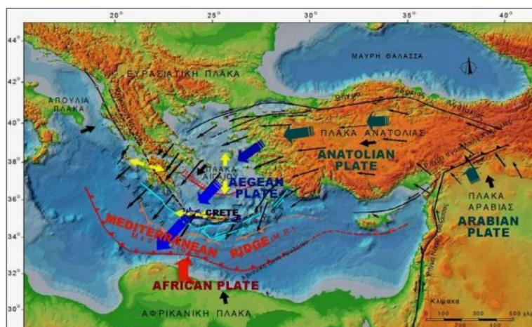
Figure 2. The geodynamic regime of the wider area of Crete and Eastern Mediterranean – The Arabian Plate pushing counterclockwise the Anatolian Plate which in turn pushes sideways the Aegean Plate; the latter overrides the African Plate which sub ducts under the island of Crete, Pavlaki, 2006.
