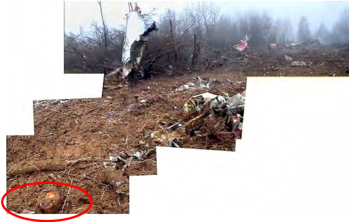
Photo 13. Unit 70A-10M of MARS-BM voice recorder on the site of crash
