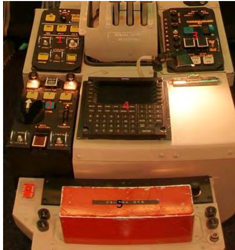
Photo 8. Panels between the pilots' seats (pedestal)
