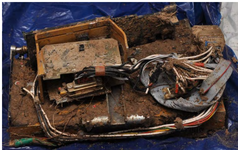
Photo 10.Quick Access Recorder ATM-QAR on the site of crash
