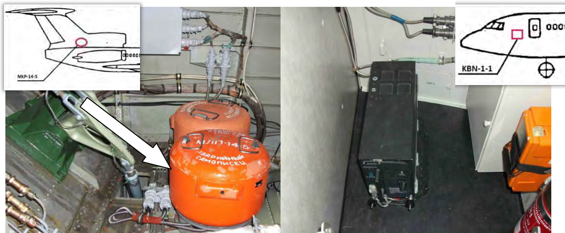
Fig. 10. Locations of crash protected flight data recorder MŁP-14-5 (left photo) and KBN-1-1 (right photo)
