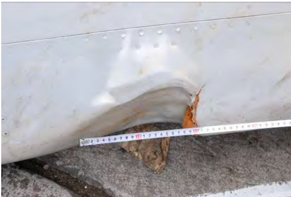
Fig. 3. Characteristic oval-shaped dents in the wing's leading edge
